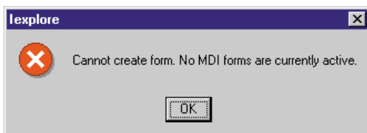
Figure 1: You receive this error message if you try to use MDI in an ActiveX control.
